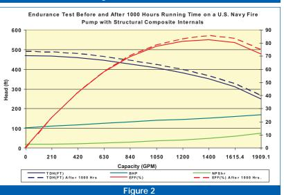
but with a shroud on the suction side of the impeller increases the efficiency of the pump by as much as 5.3 percent. It also increases the performance (flow) of the pump from 360-gpm to 400-gpm. This test was performed without any modifications to the pump and without a casing ring. If a casing ring was installed in the casing volute, the efficiency and pump performance would have increased even more.
