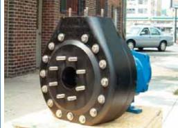
The chemical pump (for use with HCL acid) was performance tested with the open impeller and then again with an enclosed impeller. The results show a substantial improvement in efficiency and an increase in the headcapacity (H-Q) curve. The enclosed impeller would then be trimmed to the original performance specifications.
